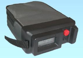
The manometer's prime function is to take accurate pressure readings of air filled telephone cables, but can also be used on other applications using non-corrosive gases. Based on a piezo-resistive sensor complete with its own laser trimmed temperature compensation, this manometer brings the user new excellence in pressure monitoring. With only two controls on the front escutcheon, the operation of the manometer is simple, quick and requires no setting time.
